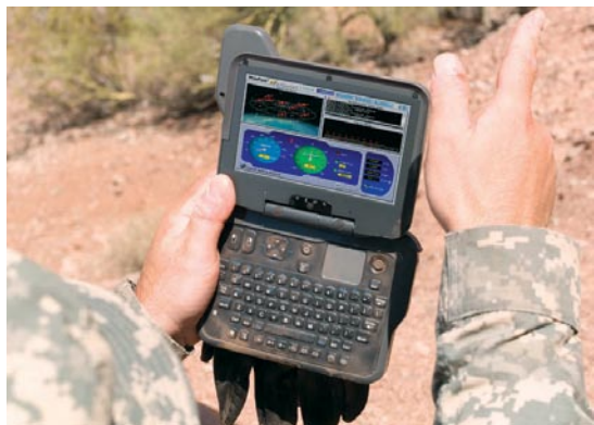
The General Dynamics Itronix GoBook MR-1 Ultra Mobile mini-laptop, which sells for $4,400. This tiny computer has GPS and numerous communications platforms built in.
